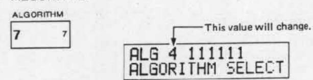
This key permits selection of one of the 32 algorithms. Press the DATA ENTRY [+1] key to increment (advance) the number of the selected algorithm, and the [-1] key to decrement the algorithm number. The slide control can be used for large variations.
