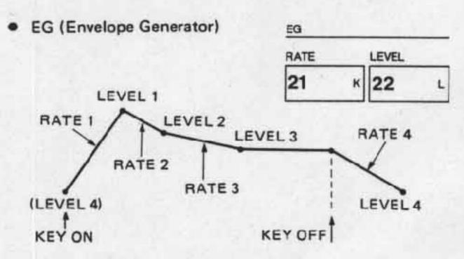
The envelope generator determines how the amplitude (volume) or timbre (tone) of a note will vary over time. Envelope modulation of a modulator results in time-based timbre variations, while envelope modulation of a carrier produces amplitude variations.
