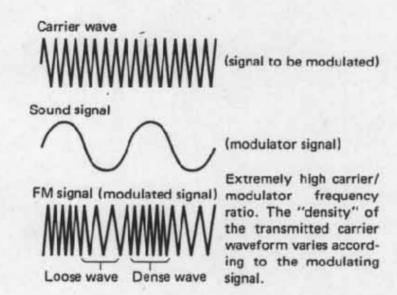
The FM tone generator system is similar in principle, but in this case both the carrier and modulator are audible signals, and their frequencies can be almost equal.
