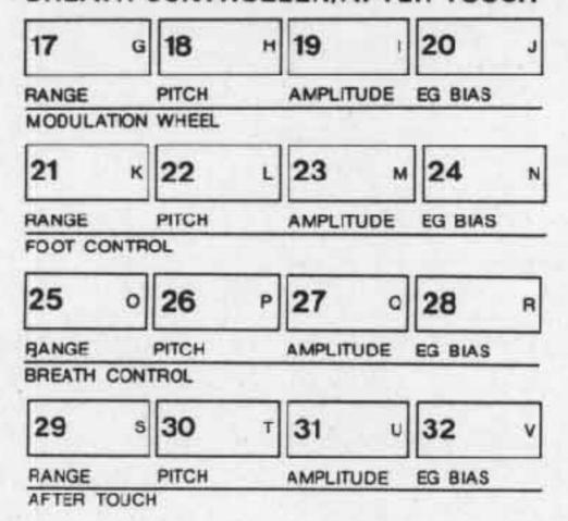
The modulation wheel, foot controller, breath controller or keyboard after touch can be used to control LFO modulation depth applied to pitch, amplitude or envelope producing controllable tremolo or vibrato effects while playing. Setting the RANGE, AMPLITUDE and ENVELOPE GENERATOR BIAS parameters for each controller is basically the same process, so we'll concentrate mainly on the MODULATION WHEEL.
